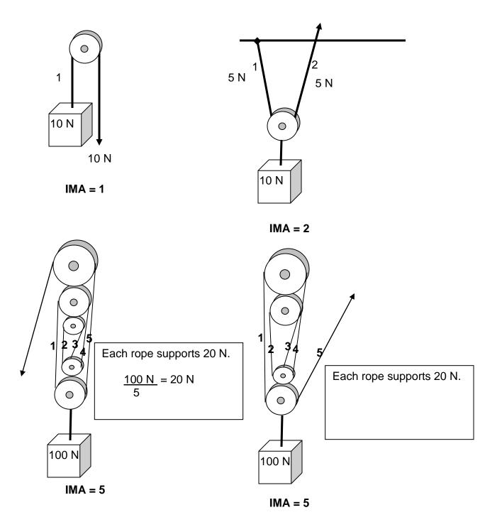
10 Determine the IMA of the following pulleys.
