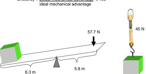
efficiency = <u>actual mechanical advantage</u> x 100 ideal mechanical advantage
