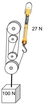
14. Determine the efficiency of the following pulley.
