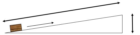
ideal mechanical advantage = <u>effort distance</u> = <u>length of ramp</u> resistance distance height of ramp 4a.. What is the IMA of this ramp? Show your work.
