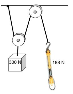
15. Determine the efficiency of the following pulley.
