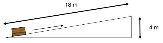
5a. To determine the AMA of the inclined plane, you must use force. The effort force is what is measured with a spring scale in Newtons. The resistance force is weight of the box in newtons.
