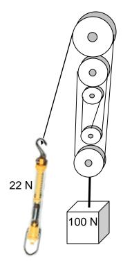
13. Determine the efficiency of the following pulley system.
